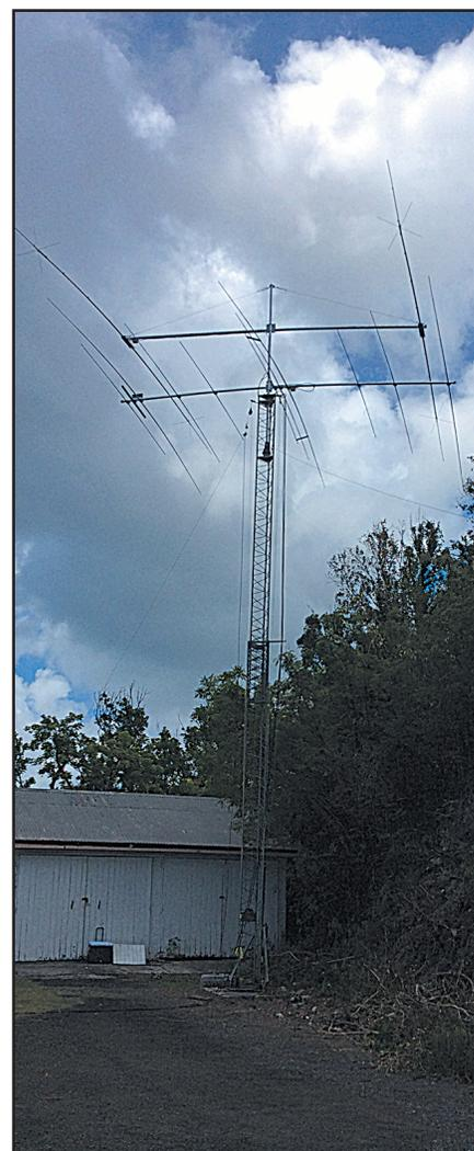
Photo F. The first post-hurricane operation from KP2M used a single 38-foot crankup tower to support an XM240, Skyhawk, and 80-meter inverted vee to make over 3,700 QSOs in single operator high power.
