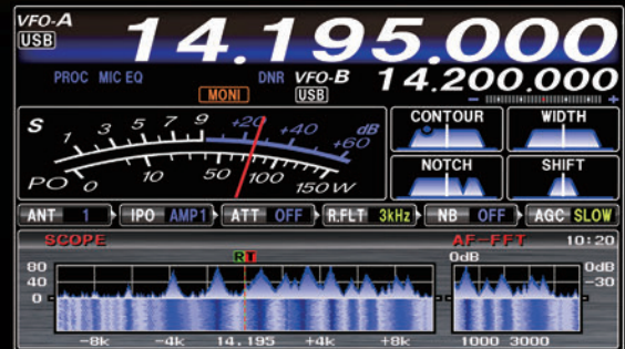
The Full Color 4.3 inch TFT display (Optional FFT-1 is required for AF-FFT Scope display.)
